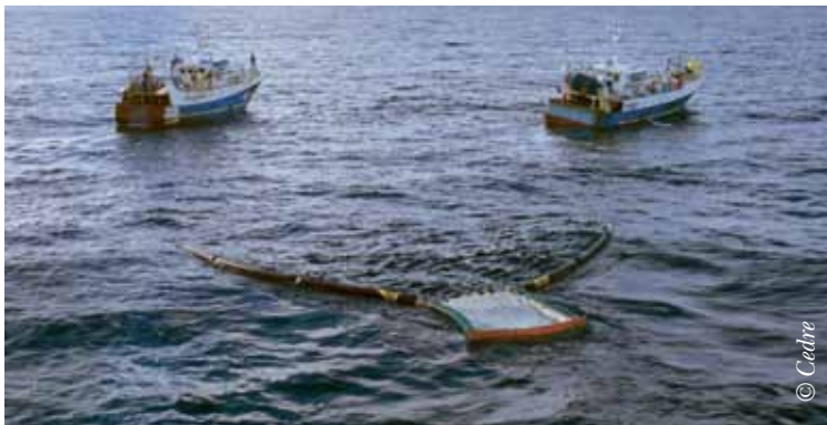
Dynamic recovery of oil using a specialised spill response trawl net
