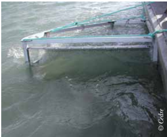
Specialised recovery equipment to facilitate the containment and manual recovery of the pollutant
