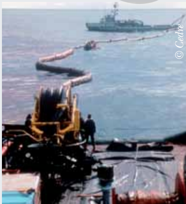
Deployment of Transrec system on board a French Navy oil spill response vessel. Sea Empress spill, Wales, 1996
