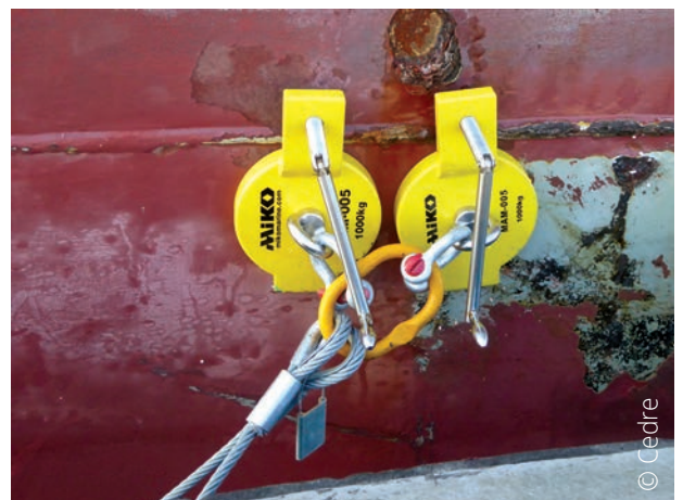
Magnetic anchoring system attached to vessel hull
