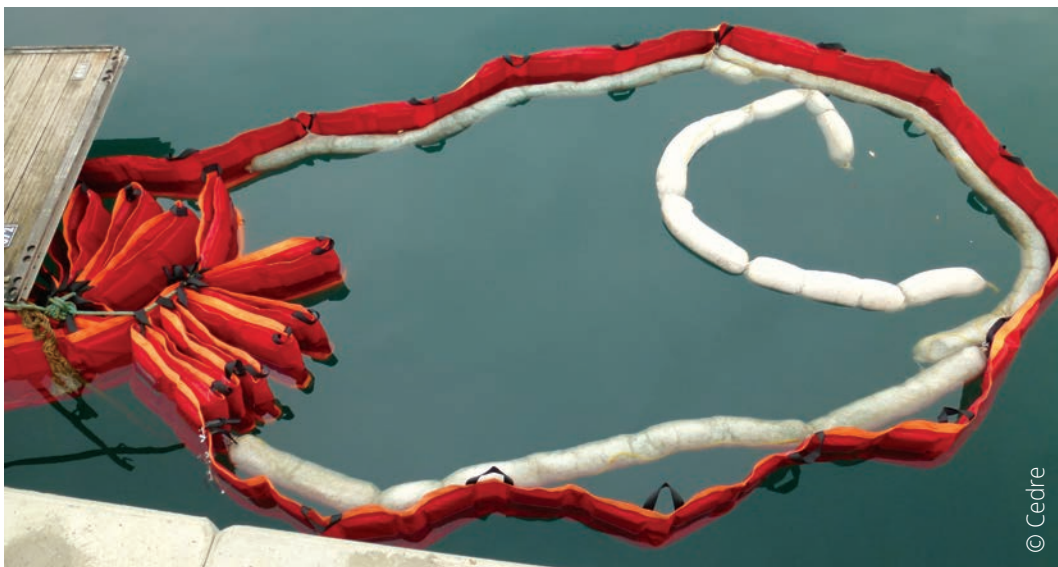
Boom moored to the wire of a tidal compensator
