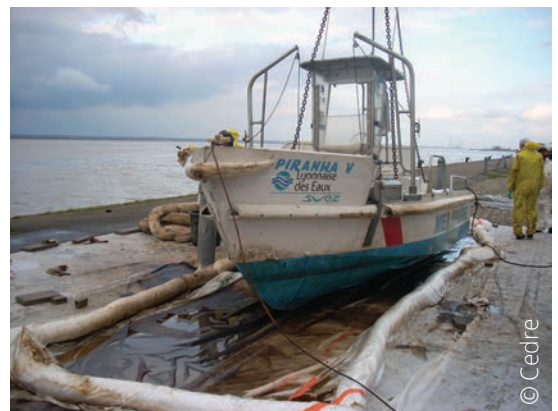
Containment area set up on shore to clean a response vessel
