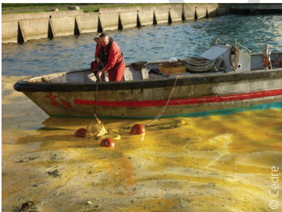
Recovering vegetable oil with a weir skimmer
