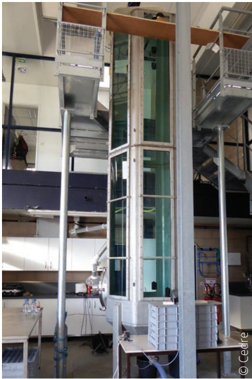
Experimental phase: releasing methane in the Cedre Experimentation Column
