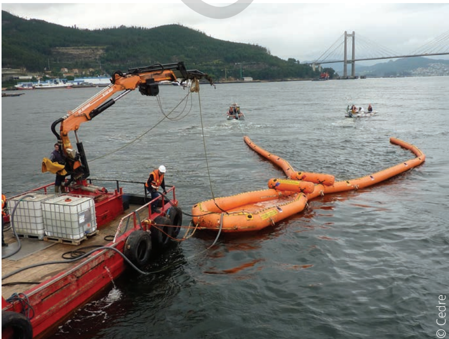
Recovery in an estuary using a recovery boom system in strong current
