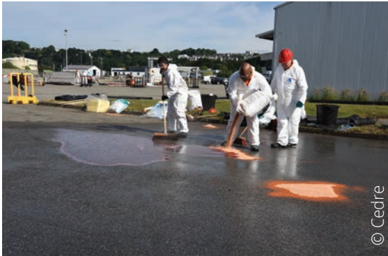
Applying bulk sorbents
