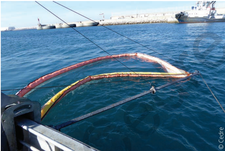
Trawling with a side beam system comprising sorbent booms arranged in series
