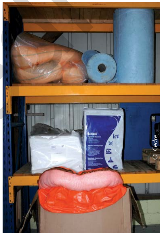
Sorbent boom, rolls, pads, bulk sorbent and sorbent boom with ballasted skirt
