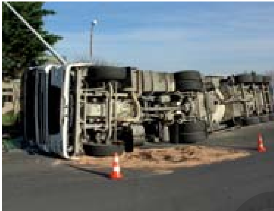
Use of sorbent on a road
