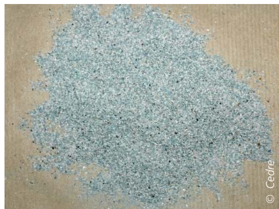
Fossilised organic universal sorbent - calcium carbonate and magnesium carbonate -
