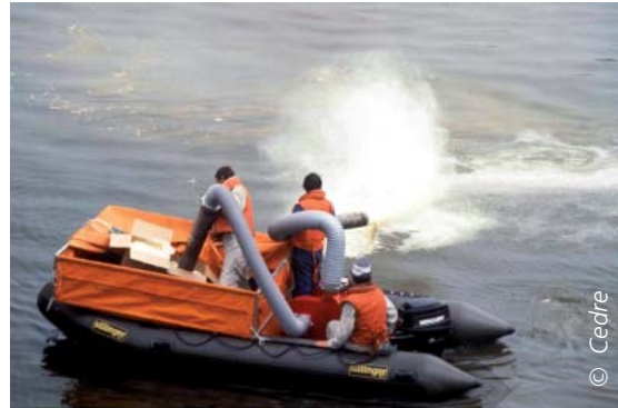
Projecting bulk sorbent onto water (right-sizing volumes of sorbent).
