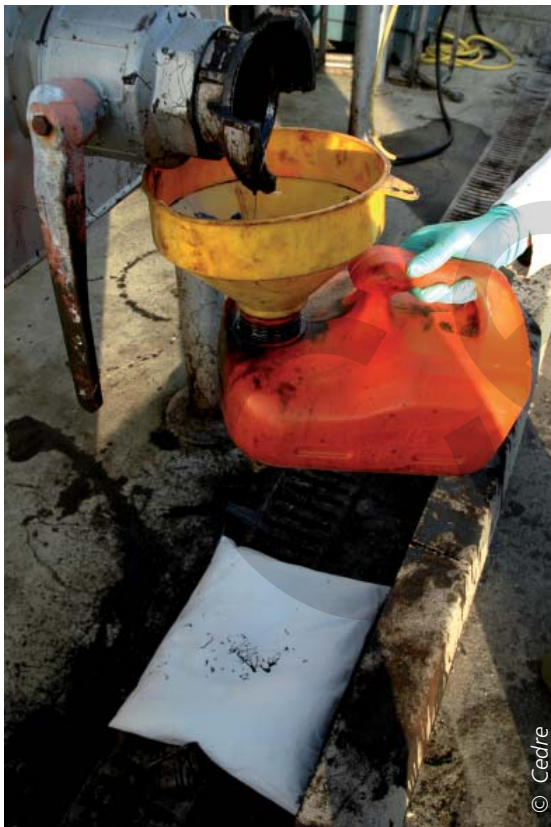
Recovery of pollutant on land using a sorbent pillow (type D)
