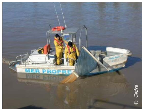
Small recovery boat using a net filled with sorbent
