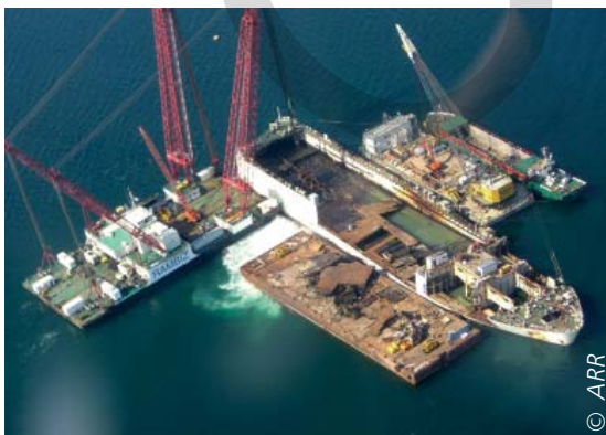
Inside of wreck cut open with sorbents deployed in addition to a skimmer
