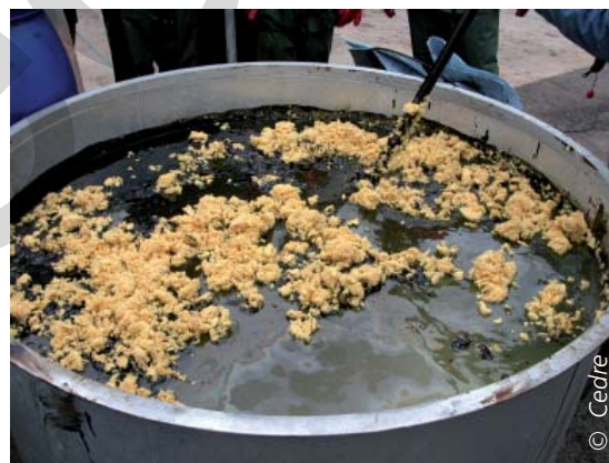
Recovery of oiled floating bulk sorbents (type A) on water
