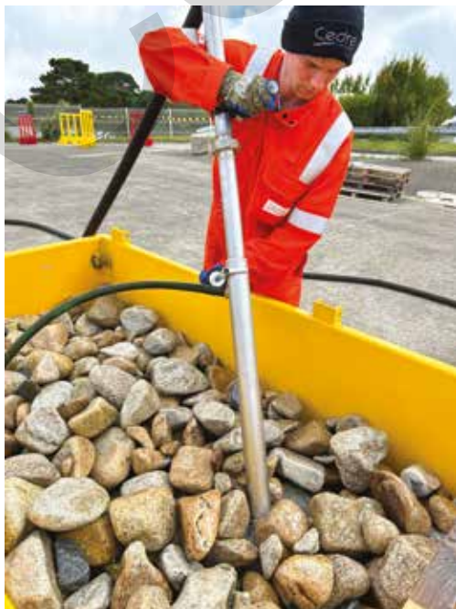
Flushing out plastic pellets trapped among pebbles.
