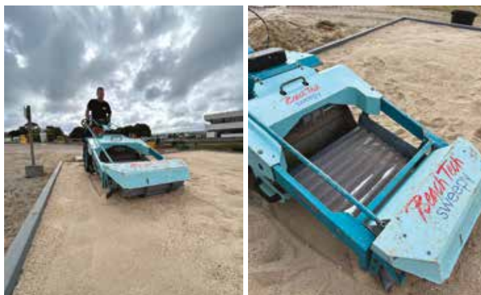
Recovering plastic pellets using a walk-behind beach cleaner.
