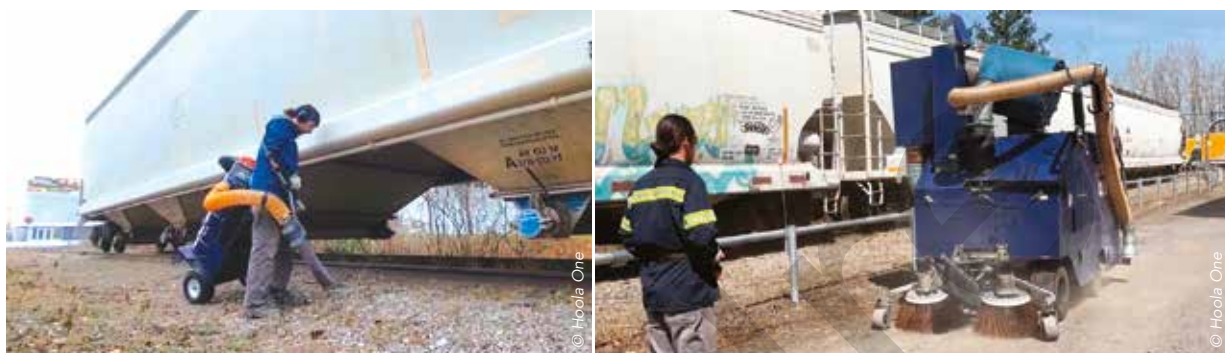
Figure 19. Example of vacuum recovery of plastic pellets on an industrial site.
