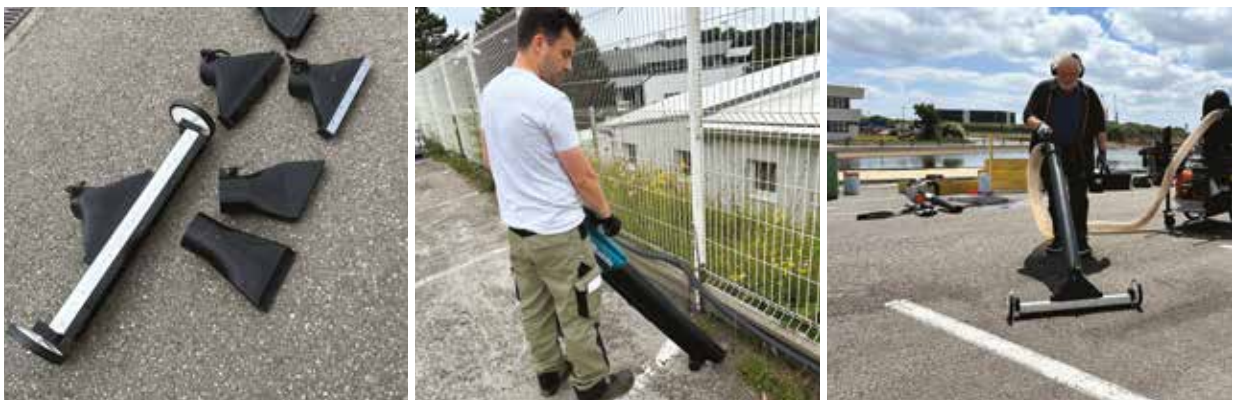
Examples of recovering plastic pellets using portable vacuum systems.
