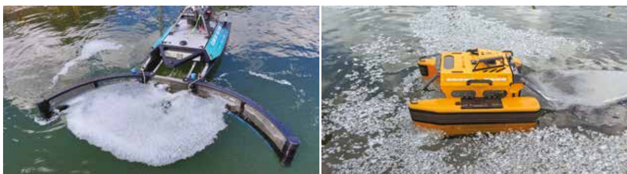
Figure 30. Recovering plastic pellets from the water surface using recovery drones controlled by a remote operator.
