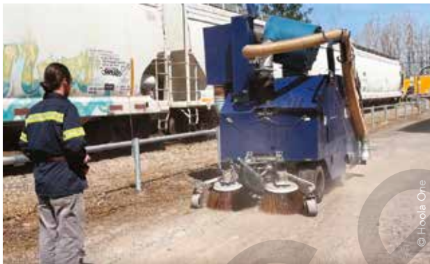
Vacuum recovery of plastic pellets on an industrial site.
