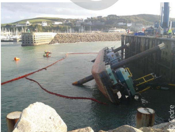
Boom deployed as a precautionary measure
