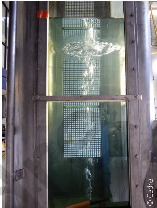
Experimental phase: releasing methane in the Cedre Experimentation Column
