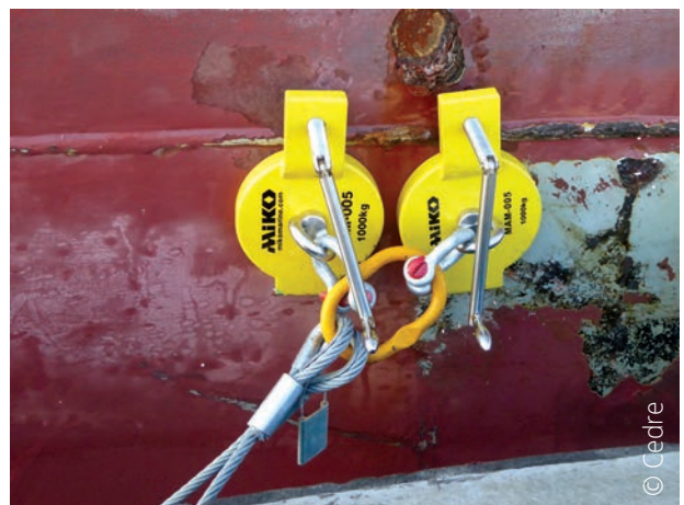
Magnetic anchoring system attached to vessel hull
