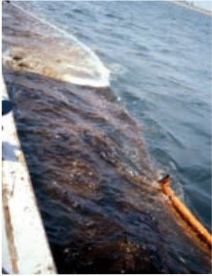
1, 2 - Dispersion trial. See the beige colour of the slick just after spraying. This effect will last once a fire monitor has jetted the oil and dispersant.
