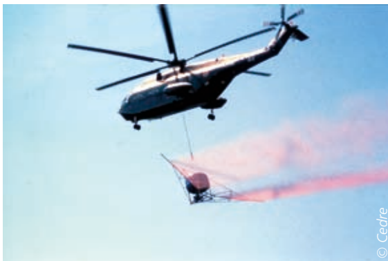
A Super Frelon heavy duty helicopter fitted with a SOKAF Bucket spraying device on location
