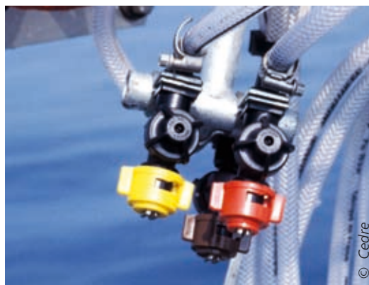
Nozzles fitted with check valves
