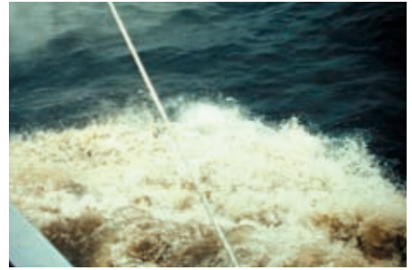
3 - Effect caused by the bow wave of a vessel passing through a treated slick. See the beige colour in the foam.
