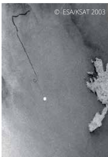
Ongoing discharge. The polluting vessel is represented by a white dot. Envisat ASAR wide swath image acquired at 20:30 UTC
