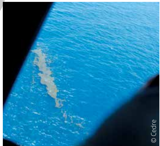
Subsequently, the films (sheen, rainbow or metallic) gradually disappear and, eventually, only patches or streaks of emulsion may remain (several days after the spill), especially in rough seas. Sheen can however reappear at a later stage, even several weeks or months after the spill, if the sea is very calm and the sun is shining.
