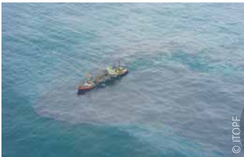
Over time, the slick fragments and the thicker areas become increasingly distinct from the thinner parts (sheen, rainbow or metallic) within a few hours to 1 day of the spill.
