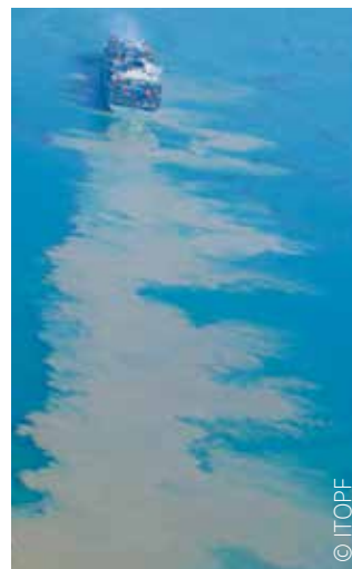
Muddy water near the coast. Silt from the seabed (muddy bottom) becoming suspended in the water due to the movement of the propellers
